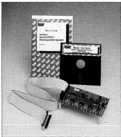
The X9241 can be used in a production environment to optimize the settings of the E 2 POT.
